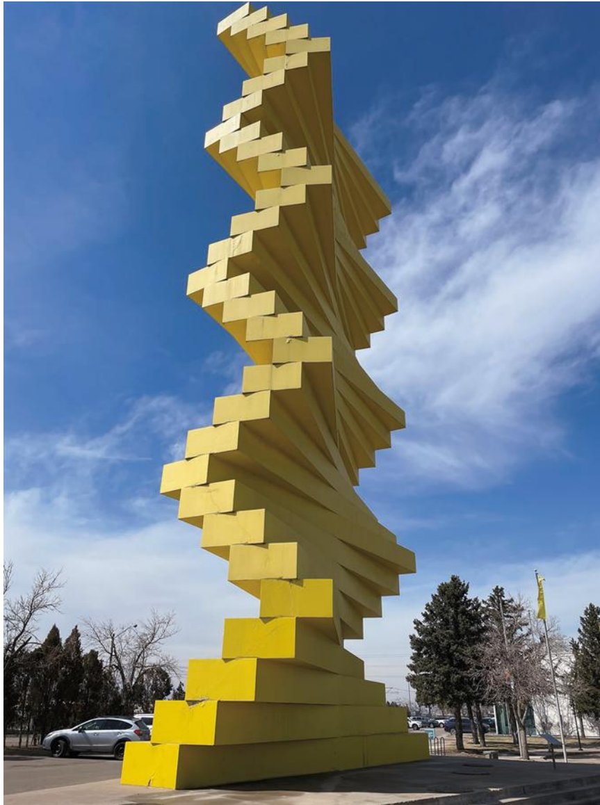
Herbert Bayer, Articulated Wall , 1985, Denver; 85 feet tall comprised of 32 prefabricated concrete pieces held together by an aircraft refueling mast in the center Photo: © Karen Foreman
